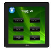
The ABtUS TP-04I is a IPS 4" LCD touch screen panel with a resolution of 480x480 pixels.
